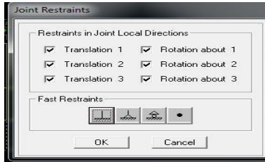
Gambar 2.8 Kotak joint restraints
